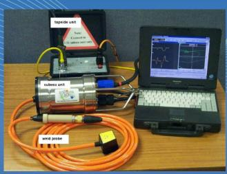
U31D Crack Micro Gauge System (with short test umbilical)
