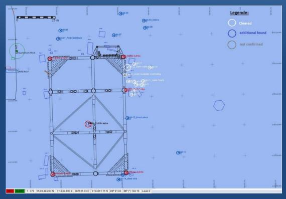
Logged target positions to support the divers and ROV's clearance tasks. After an initial survey additional targets identified can be added. The work progress can be monitored and documented. An as left survey of located targets is more simply and faster.
