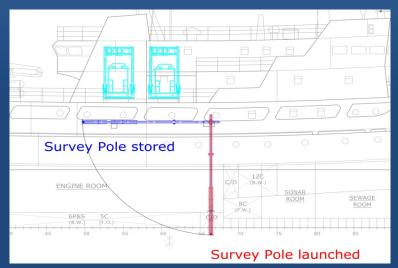
In lowered position, the flange of the pole is located approx. 0,5m under the keel of the vessel. Draught of the vessel is approx. 4,6m.
