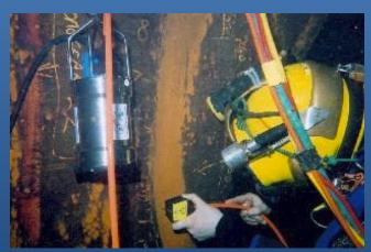
Diver uses the U31D Crack Micro Gauge System
