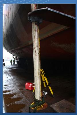
Bracket mounted at the DSV RS Sentinel's keel blade to prevent vibrations. The bracket can be installed by our diving team in port or at sea.
