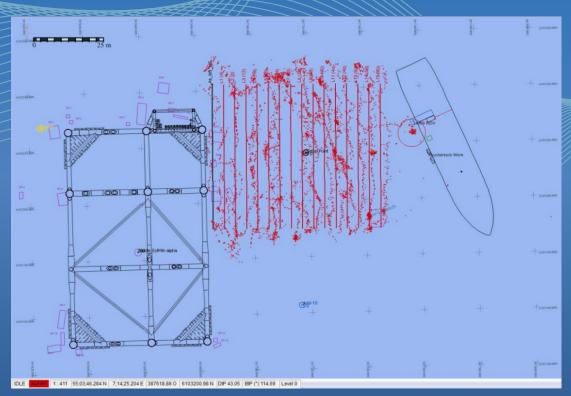
Logged positions of an ROV video inspection across survey lines to ensure a 100% coverage along the required survey area.
